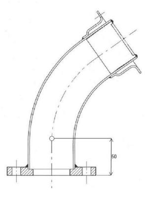
Please note that it will be possible to fit the exhaust probe to the old manifolds as well, respecting the above-mentioned dimensions.
